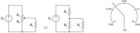
The position of the wiper determines the output voltage of the potentiometer. Your potentiometers may vary. You should consult the datasheet of your potentiometer for detailed specifications.
