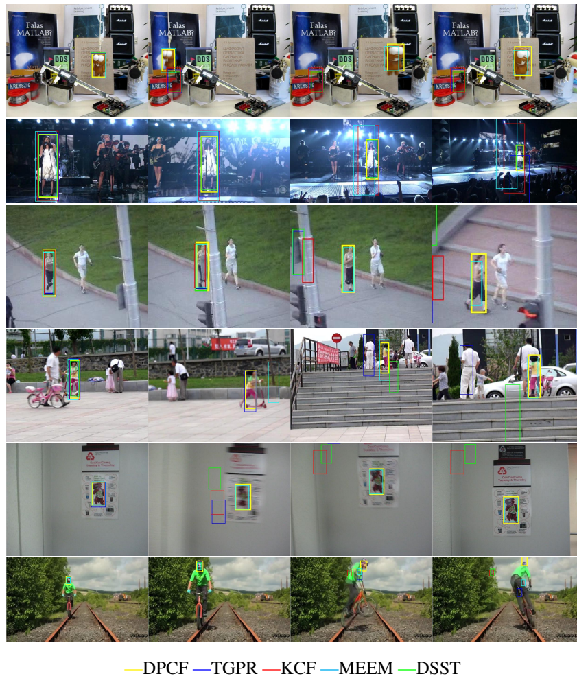
Figure 7: DPCF tracker compared with the top 5 methods that include TGPR [17], MEEM[18], DSST [12] and KCF [4] showed in challenging frames i.e., occlusions, deformation, illumination variations and scaling. The sample sequences are from the Lemming , Singer1 , Jogging-1 , Girl2 , BlurOwl and Biker [33] respectively. Our method handles occlusion and scale changes more accurately than the other trackers.
