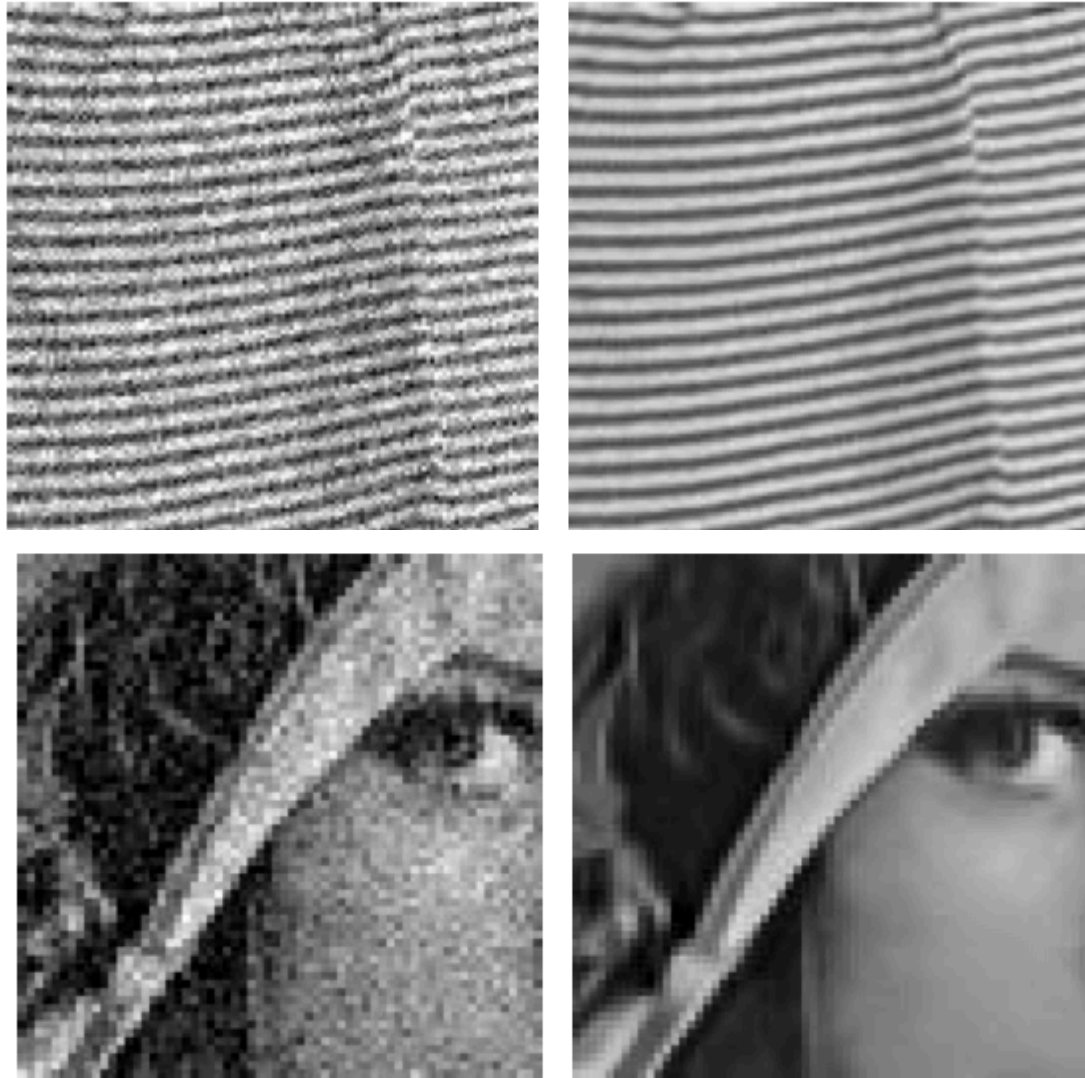
FIG. 9. NL-means denoising experiment with a natural image. Left: Noisy image with standard deviation 20. Right: Restored image.
