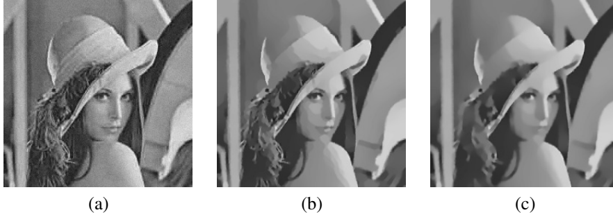
Figure 2: The staircasing effect. (a) Original noisy image. (b) Perona-Malik diffusion. (c) Regularized Perona-Malik diffusion.
