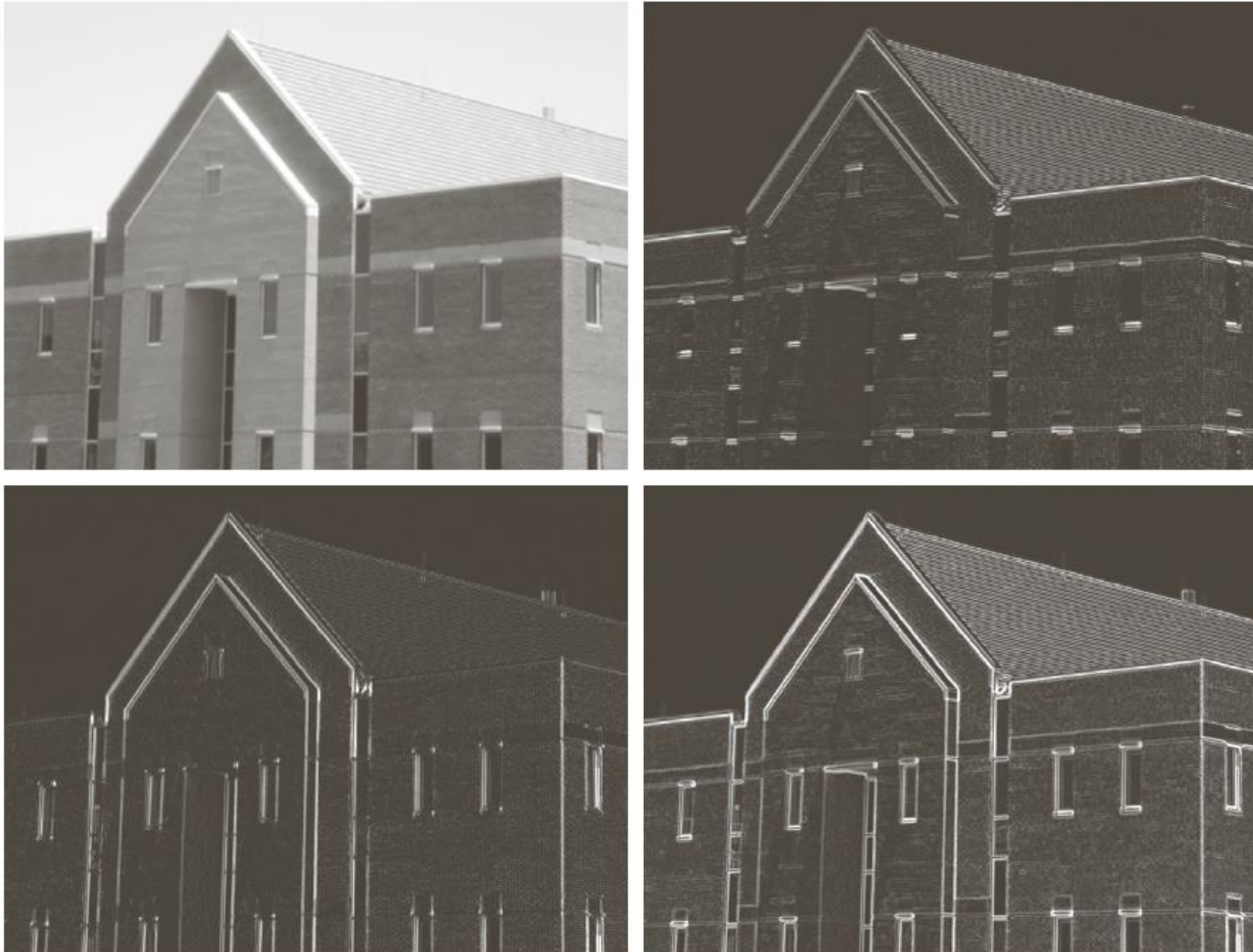
FIGURE 10.18 Same sequence as in Fig. 10.16, but with the original image smoothed using a 5 \times 5 averaging filter prior to edge detection.
