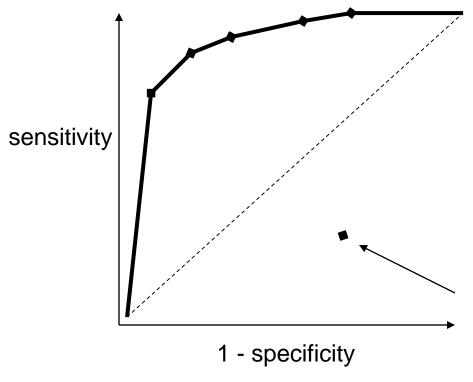
All the optimal detectors lie on the convex hull.
