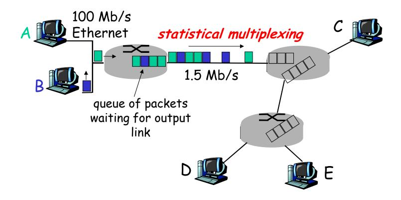
Sequence of A & B packets does not have fixed pattern, bandwidth shared on demand  $\Rightarrow$  statistical multiplexing. TDM: each host gets same slot in revolving TDM frame.
