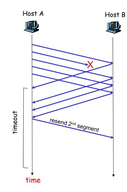
Figure 3.37 Resending a segment after triple duplicate ACK Layer 3-72
