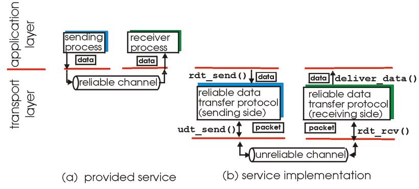
characteristics of unreliable channel will determine complexity of reliable data transfer protocol (rdt)
