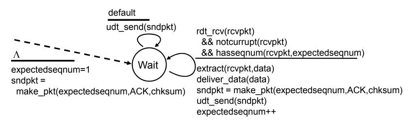
ACK-only: always send ACK for correctly-received pkt with highest *in-order* seq #
