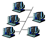
shared wire (e.g., cabled Ethernet)
