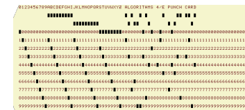
punch card (12 holes per column)
