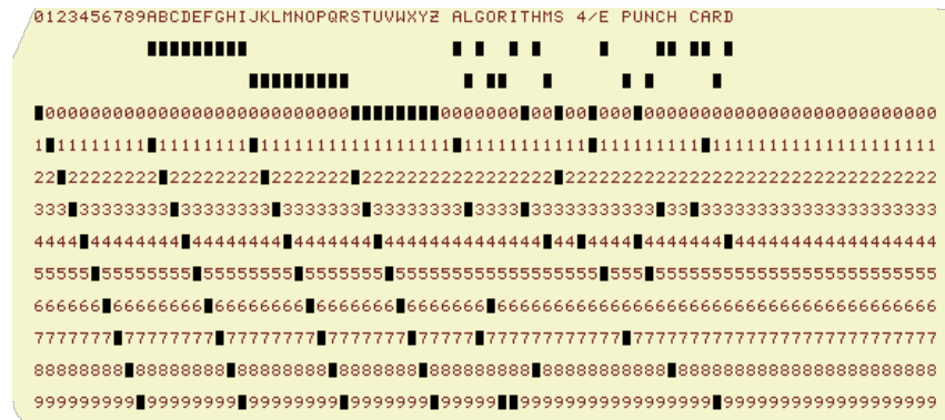
punch card (12 holes per column)
