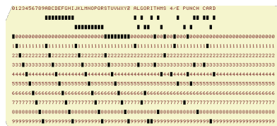
punch card (12 holes per column)
