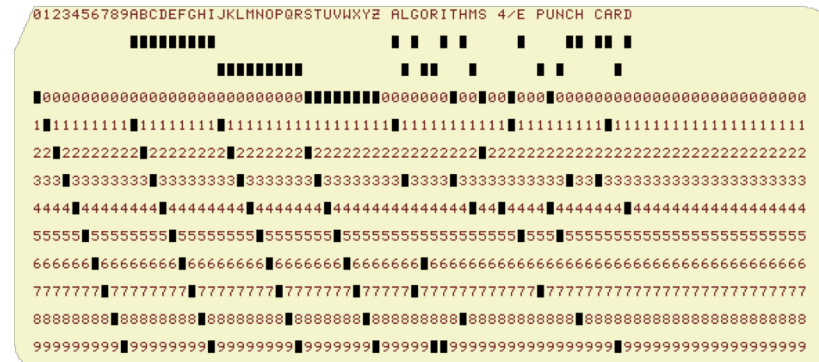
punch card (12 holes per column)
