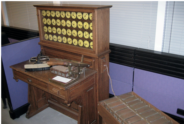
Hollerith tabulating machine and sorter
