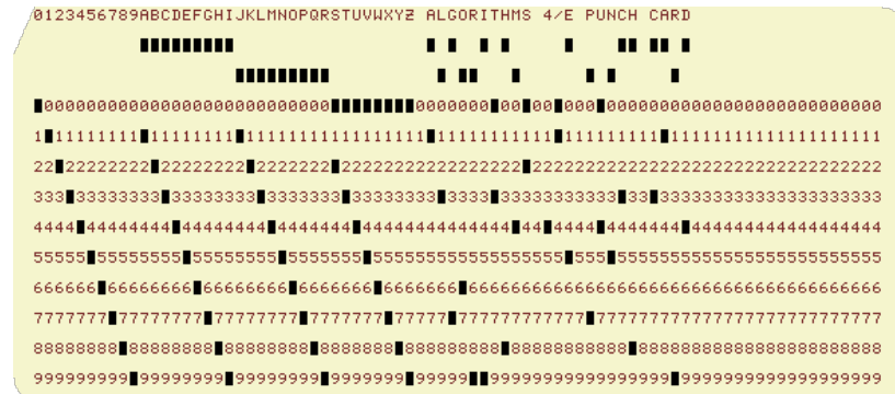
punch card (12 holes per column)
