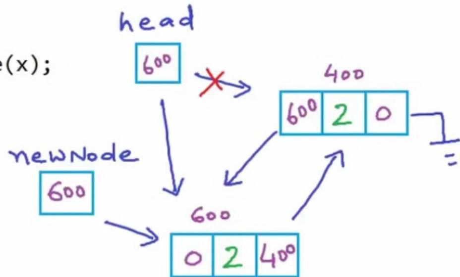
Set the **prev-field** of the **head** node as 600 (address of the new node).
