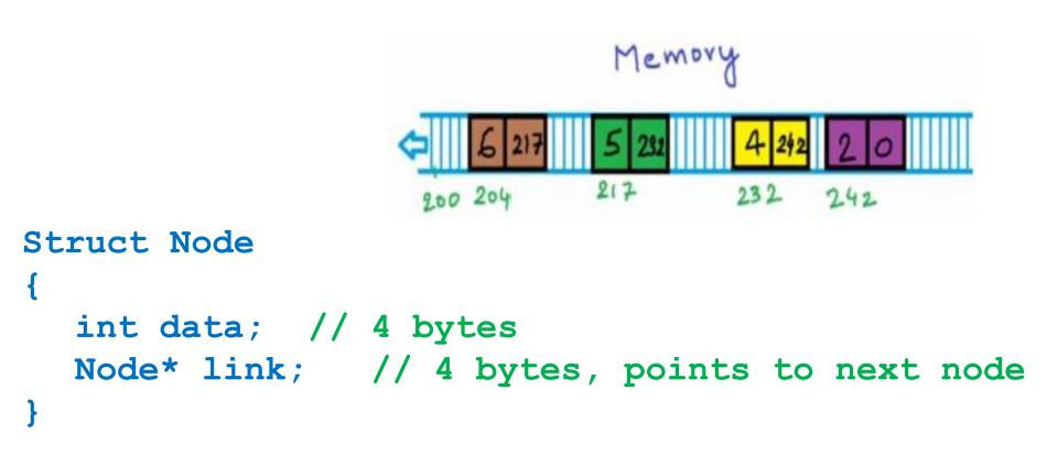
For each element (or node) two fields are stored, each costing four bytes.
