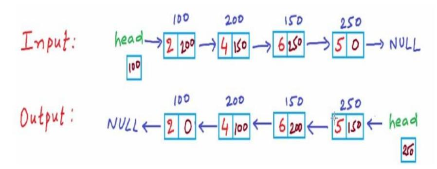
Links should be changed. Head node should point to the node at address 250. For the first node, we cut the link from head and build a link to NULL.
