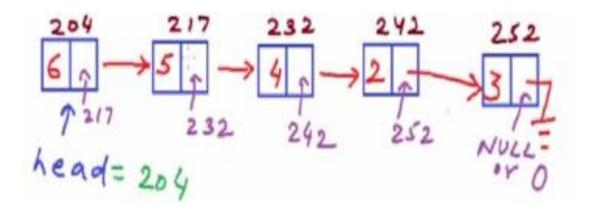
Create a node independently with some memory location and adjust the links properly. Say the node 3 gets address 252.
