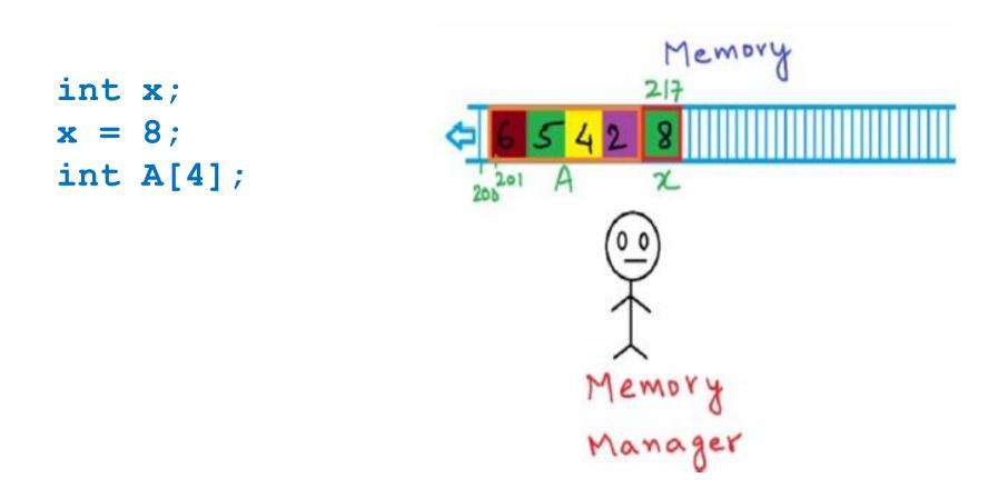
An array is stored as one contiguous block of memory. How can we add a fifth element to the array A above???
