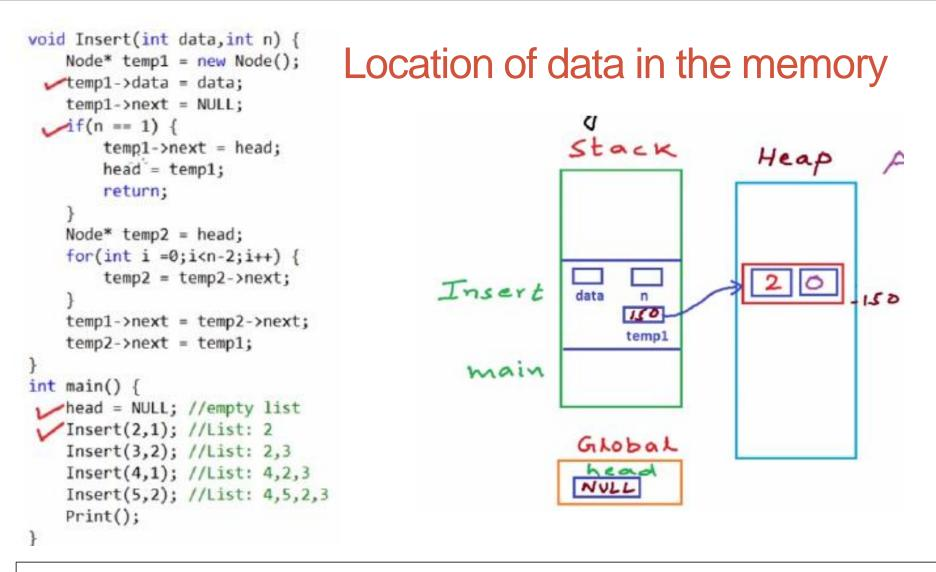
When we store something in the heap using **new** or **malloc**, we do not have a variable name for this and we can only access it through a pointer variable as seen above.
