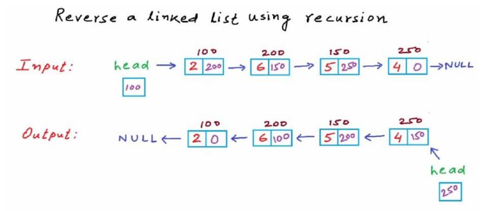
The address passed to the reverse function is the address of the first node. As soon as we reach the last node, the program modifies the head pointer to point to the fourth node.
