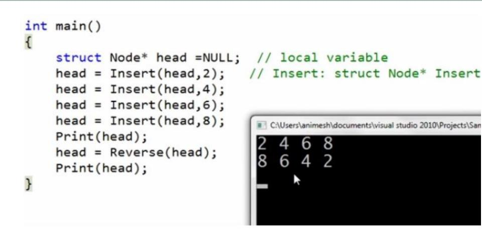
The insert function takes two arguments: the address of the head node and the data to be inserted.
