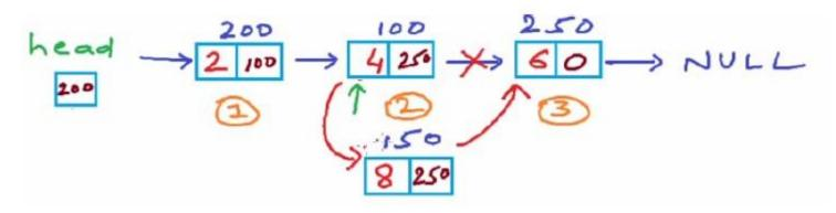
Say, we want to insert a value 8 at 3rd position. The link field of the new node should be 250 and the link field of the second node should be the address of the new node as shown below.
