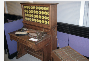
Hollerith tabulating machine and sorter
