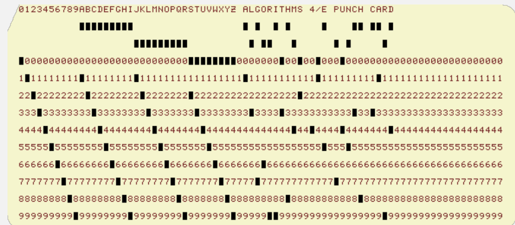
punch card (12 holes per column)
