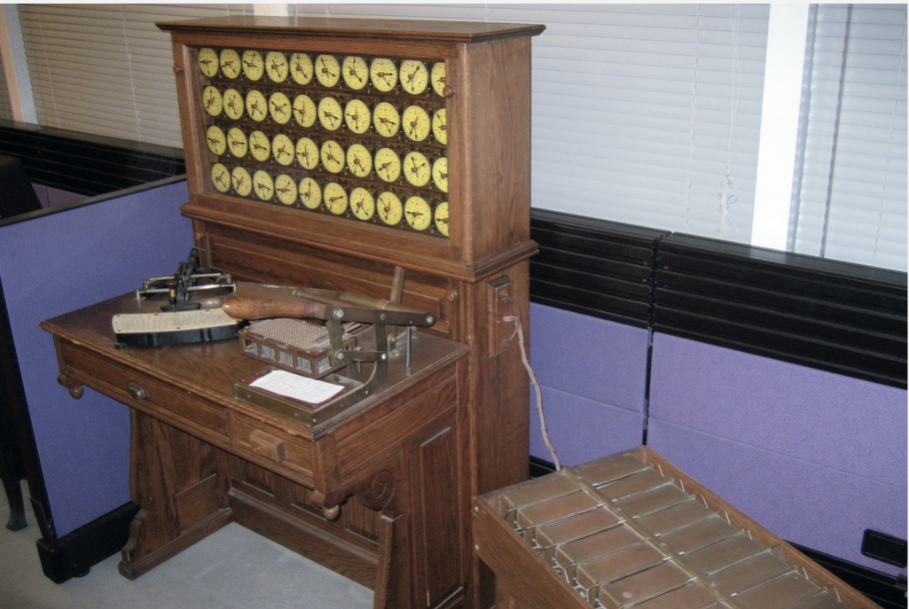
Hollerith tabulating machine and sorter
