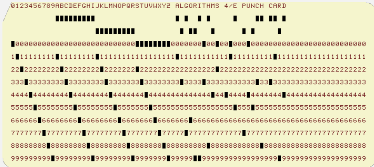
punch card (12 holes per column)
