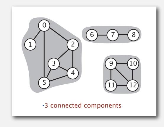
connected component id (easy to compute with DFS)
