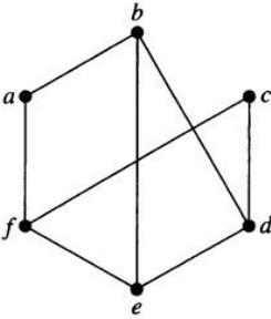
**Solution:** The first graph is bipartite, since it has a proper 2-coloring by using color red on  $\{a, b, e, d\}$  and color blue on  $\{c, f\}$ . The second graph is not bipartite, since there is a triangle on the vertices  $\{b, d, e\}$  and we cannot 2-color a triangle properly.
