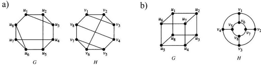
**Solution:** In part (a), the graphs are isomorphic. Let the isomorphism function  $f$  be defined as,  $f(u_1) = v_2$ ,  $f(u_2) = v_3$ ,  $f(u_3) = v_1$ ,  $f(u_4) = v_8$ ,  $f(u_5) = v_4$ ,  $f(u_6) = v_5$ ,  $f(u_7) = v_7$ ,  $f(u_8) = v_6$ .
