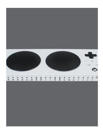
Microsoft's Xbox Adaptive Controller makes gaming on Xbox One consoles and Windows 10 PCs more accessible for players with limited mobility. Its two large programmable buttons and 19 jacks empower players to connect additional switches, joysticks, and other assistive devices to customize the way they play their favorite games.
