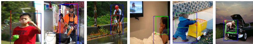
Fig. 2. The first three images show the person bounding boxes and the face detector outputs, and the latter ones shows face regions determined wrt person bounding boxes.
