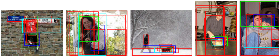
Fig. 3. An example execution of the MIL framework (best viewed in color). Amongst the 10 example object regions extracted by [5] from the training set, the top 3 regions that contribute to the classification are shown in green, cyan and blue respectively.
