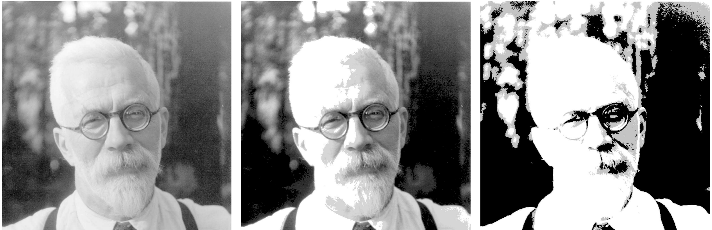
FIGURE 14.9. Sir Ronald A. Fisher (1890 – 1962) was one of the founders of modern day statistics, to whom we owe maximum-likelihood, sufficiency, and many other fundamental concepts. The image on the left is a 1024 \times 1024 grayscale image at 8 bits per pixel. The center image is the result of 2 \times 2 block VQ, using 200 code vectors, with a compression rate of 1.9 bits/pixel. The right image uses only four code vectors, with a compression rate of 0.50 bits/pixel
