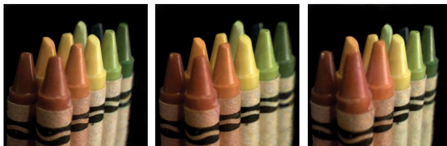
Shifts in point of view are another option in images made with Ng’s light-field camera. All three images come from a single exposure, but the camera seems to move laterally, and in the rightmost panel is brought closer to the subject. (Images courtesy of Ng.)
