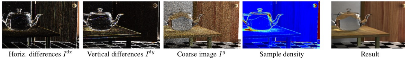
Figure 1: We compute image gradients I^{dx} , I^{dy} and a coarse image I^g using a novel Metropolis algorithm that distributes samples according to path space gradients, resulting in a distribution that mostly follows image edges. The final image is reconstructed using a Poisson solver.
