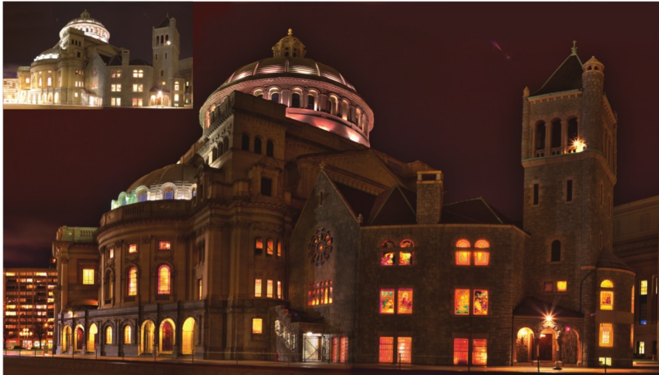
Figure 1: The bilateral grid enables edge-aware image manipulations such as local tone mapping on high resolution images in real time. This 15 megapixel HDR panorama was tone mapped and locally refined using an edge-aware brush at 50 Hz. The process used about 1 MB of texture memory. The inset shows the original input.
