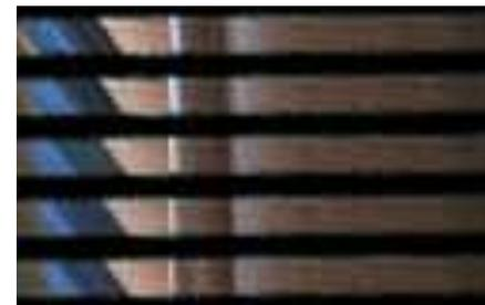
Characteristic behavior: points in scene become lines with slope depending on distance. Objects at focus plane produce vertical features; more distant objects produce negative slopes.
