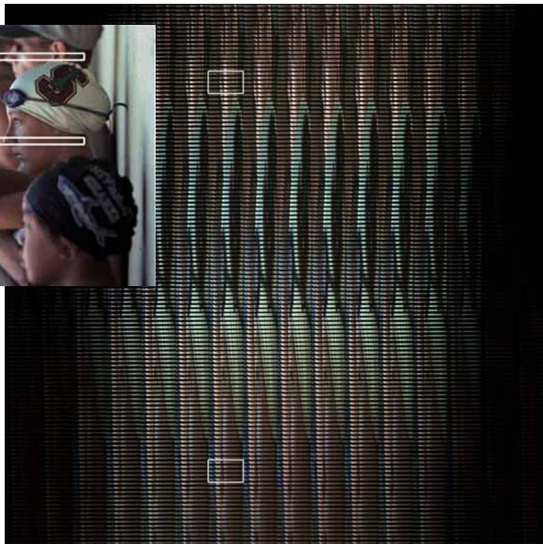
Epipolar plane format:  $(v,t)$  is the outer loop and  $(s,u)$  is the inner loop.
