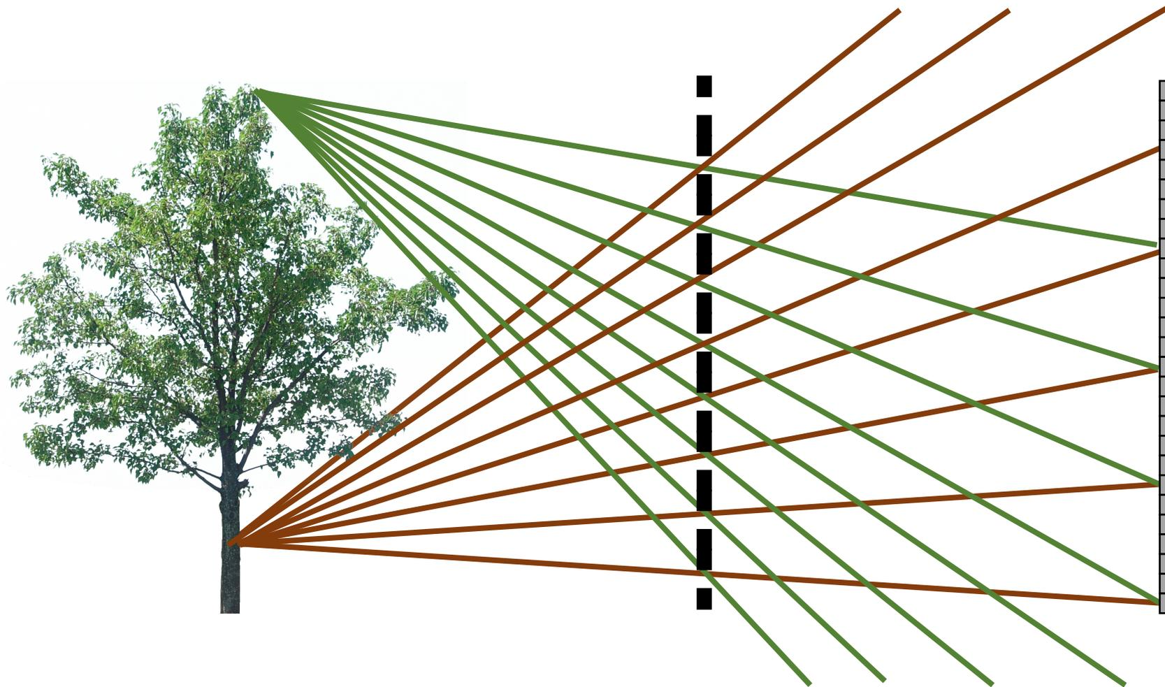
Need to be able to separate different rays falling on same pixel.
