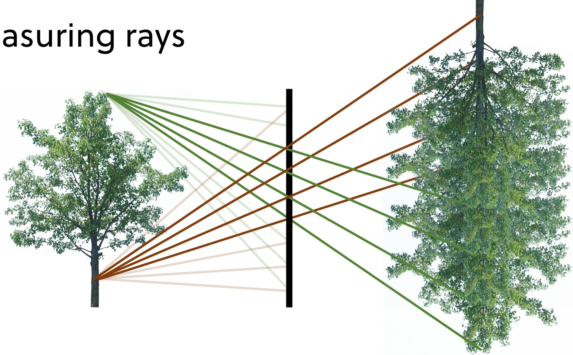
We can capture the same set of rays by using a pinhole camera from multiple viewpoints
