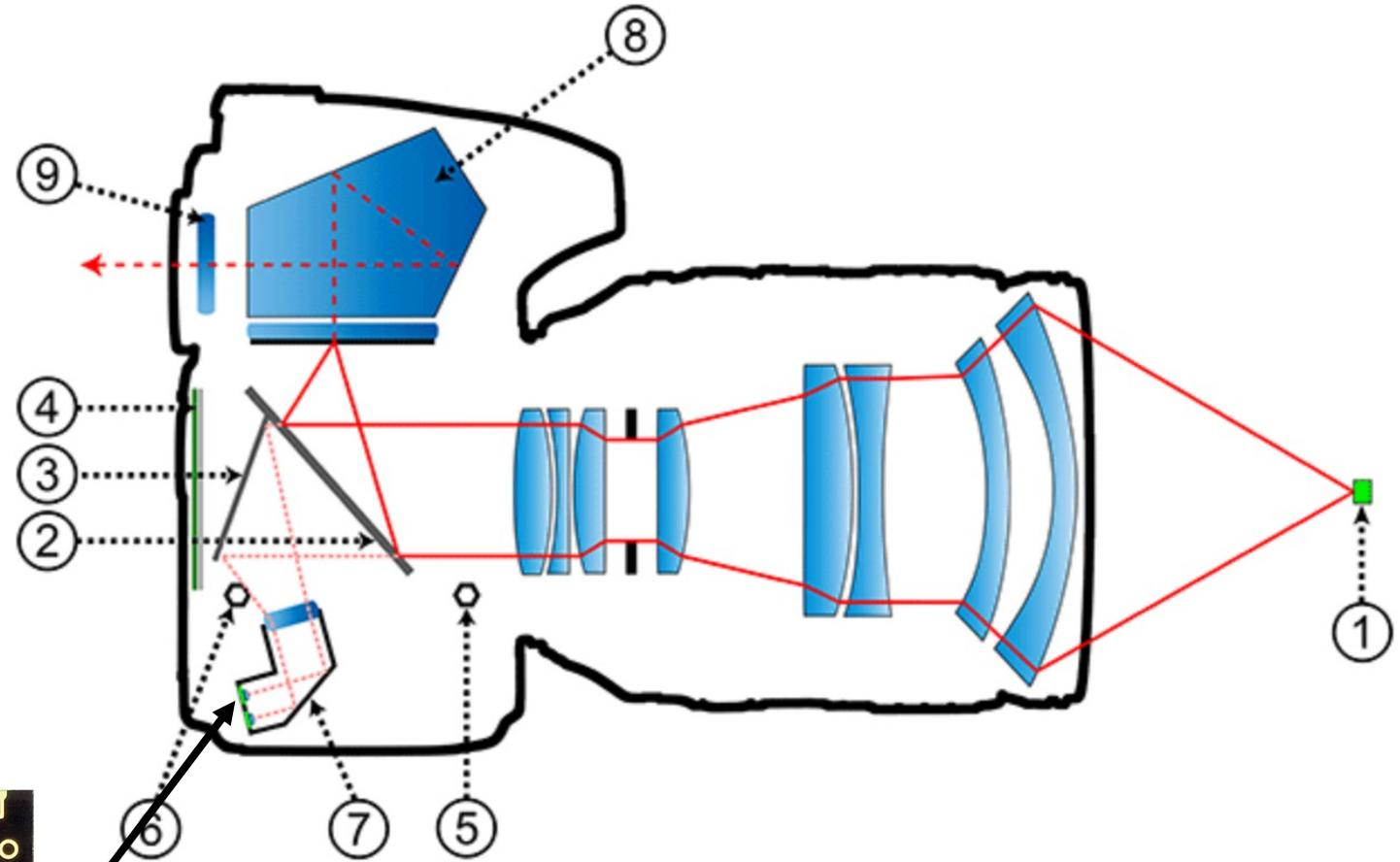
DSLR mirror has a translucent part that allows some light to make it to the AF sensor.
