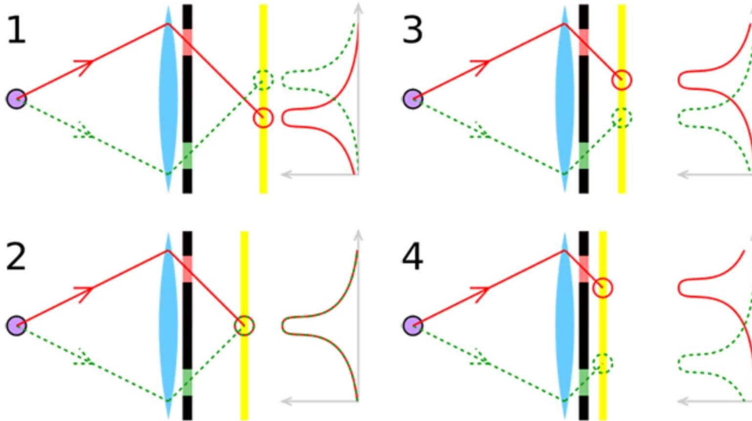
Each yellow box indicates two sensors, each measuring light from different parts of the aperture.
