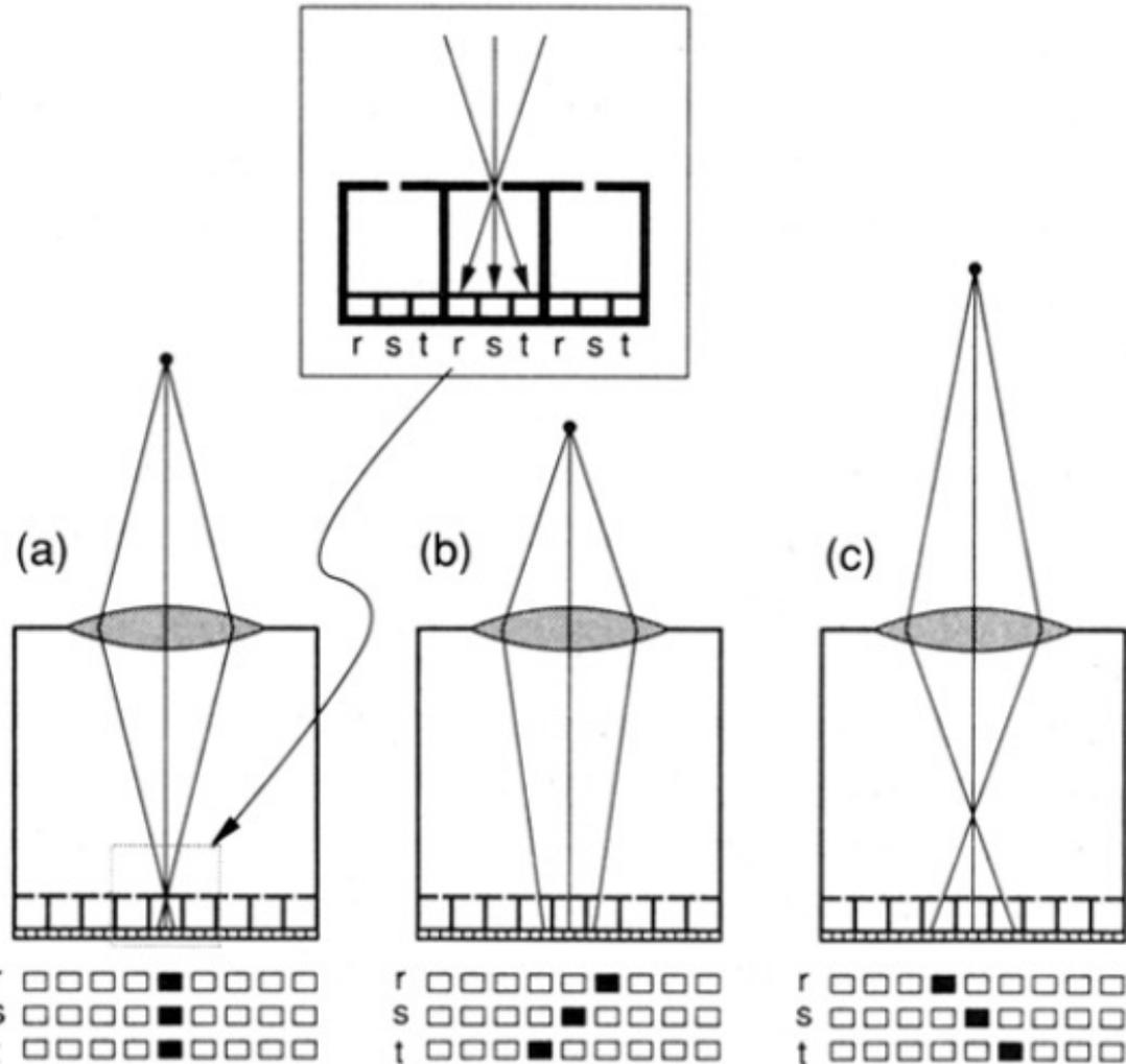
Figure from the 1992 paper, which shows the version of the plenoptic camera with pinholes instead of lenslets on the image plane.
