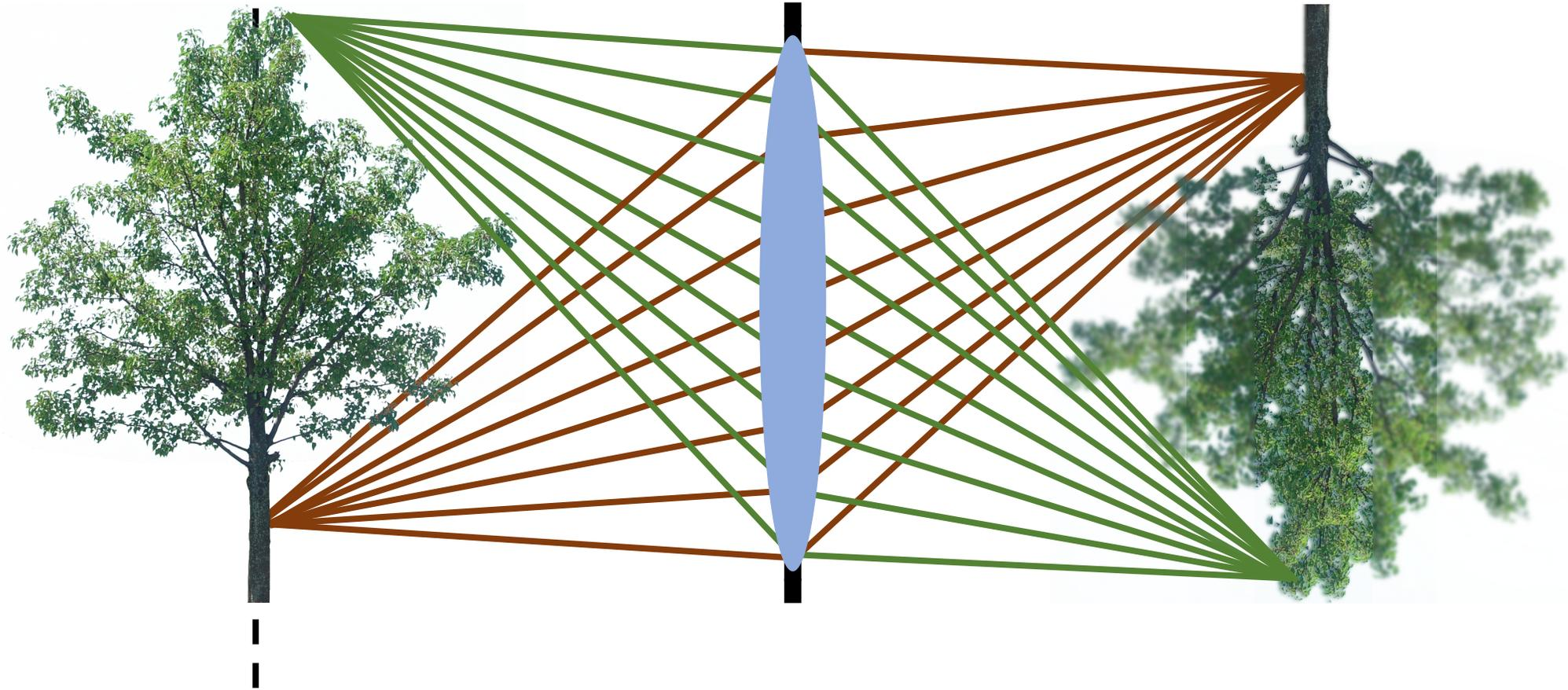
A lens measures all rays radiated from the object (up to aperture size).
