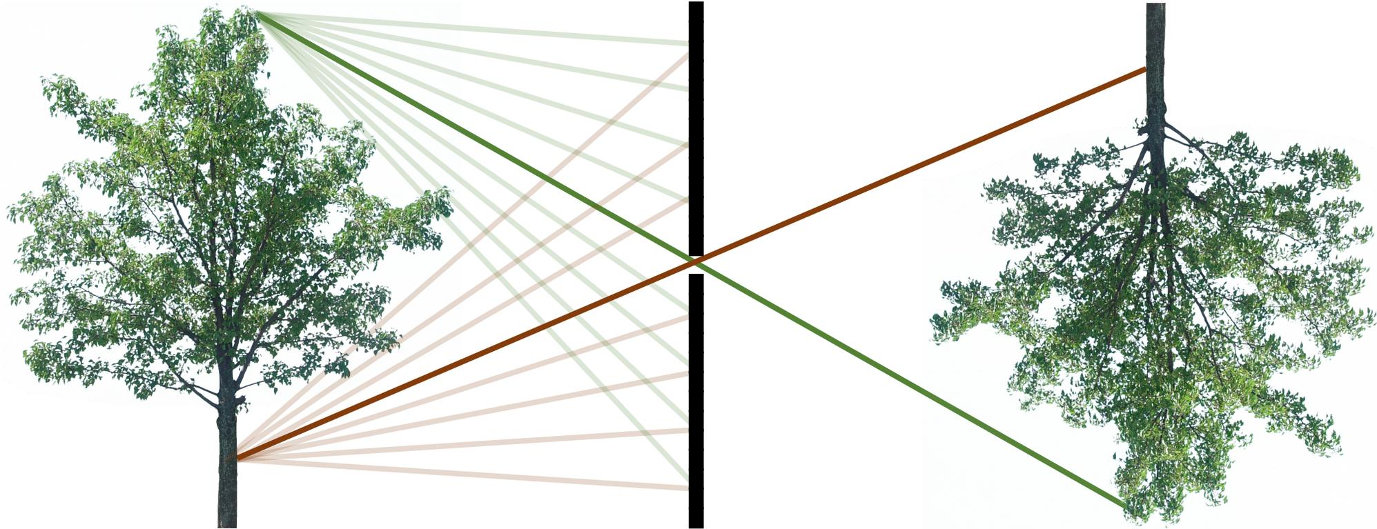
We can capture the same set of rays by using a pinhole camera from multiple viewpoints
