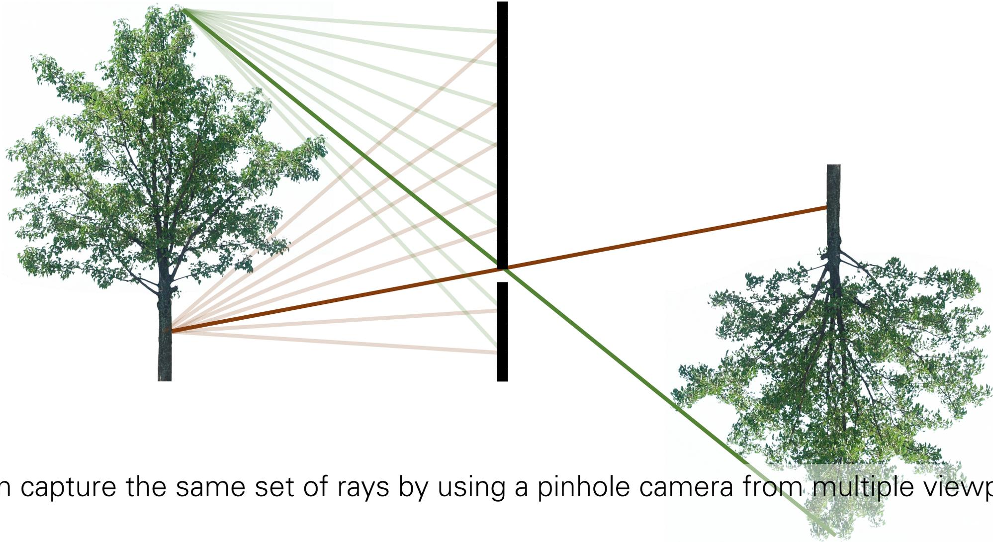
We can capture the same set of rays by using a pinhole camera from multiple viewpoints
