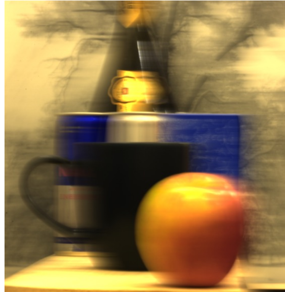
parabolic input - blur is invariant to velocity
