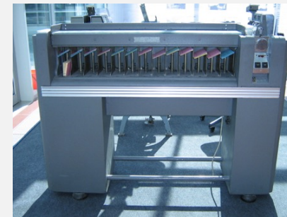
IBM 80 Series Card Sorter (650 cards per minute)
