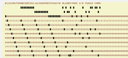
punch card (12 holes per column)
