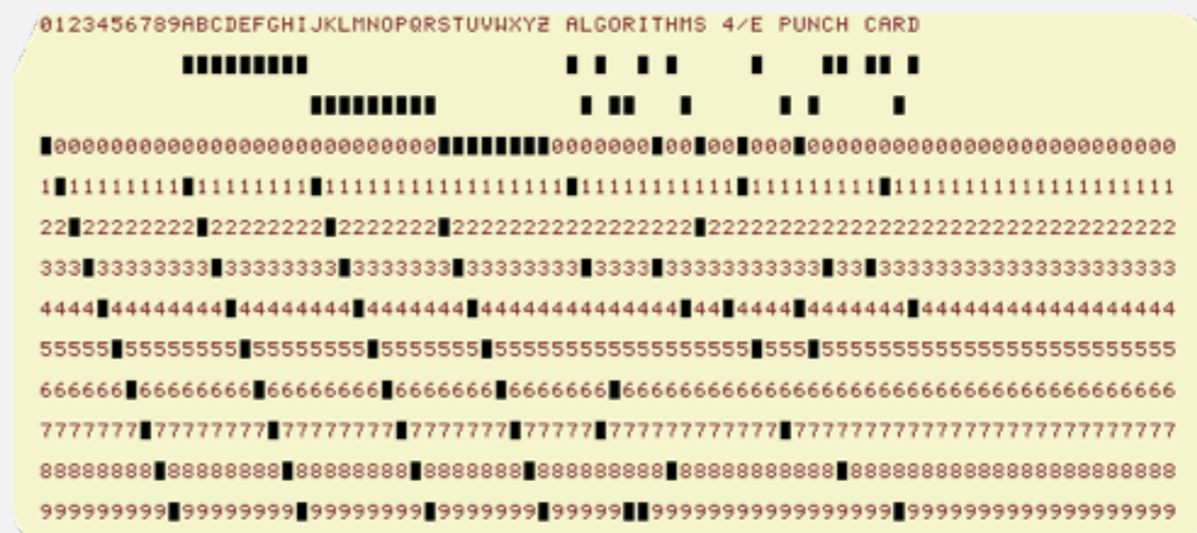
punch card (12 holes per column)
