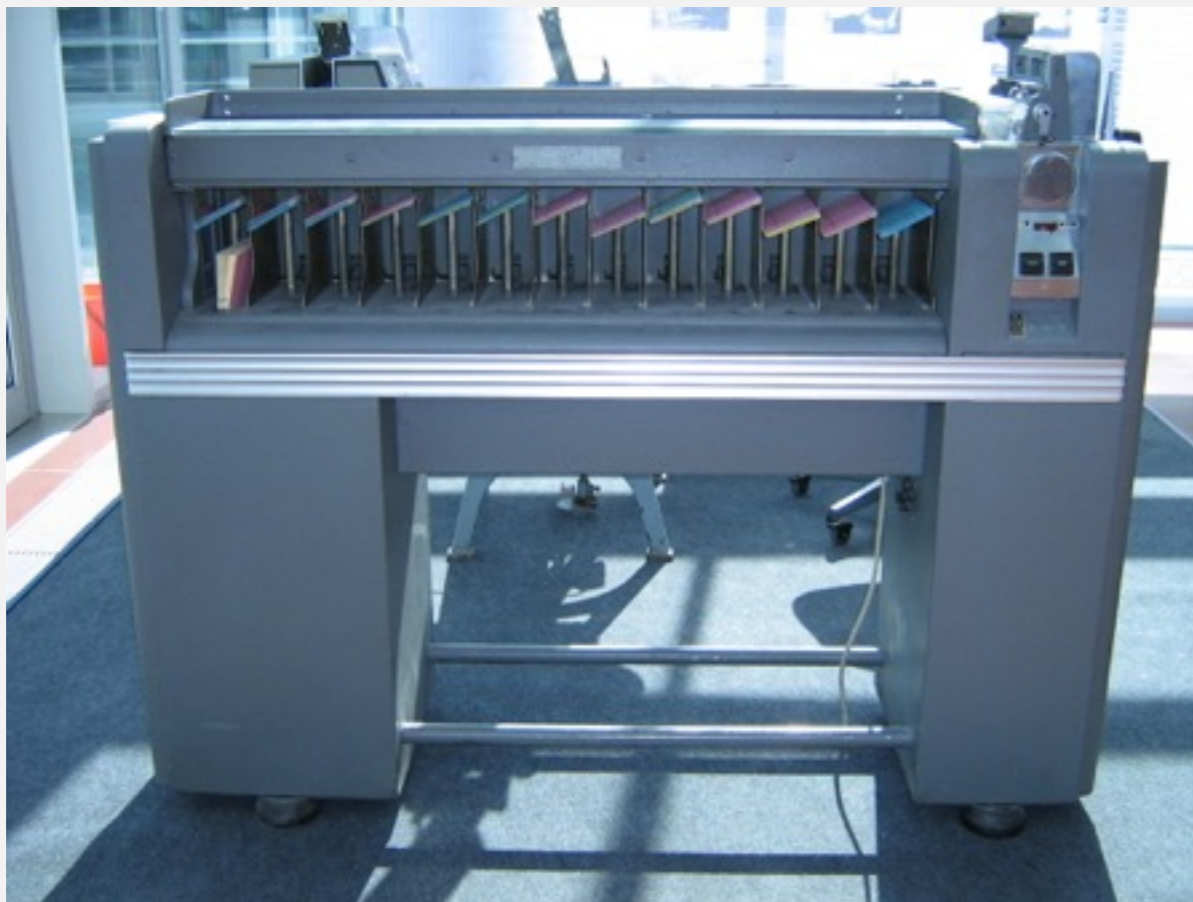
IBM 80 Series Card Sorter (650 cards per minute)
