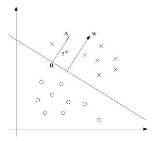
The decision boundary corresponding to (w, b) is shown, along with the vector w. Note that w is orthogonal (at 90°) to the separating hyperplane. (You should convince yourself that this must be the case.) Consider the point at A, which represents the input  $x^{(i)}$  of some training example with label  $y^{(i)} = 1$ . Its distance to the decision boundary,  $\gamma^{(i)}$ , is given by the line segment AB.
