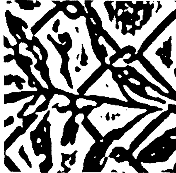
convolution with \nabla^2 h_\sigma(u, v) pos. values – white neg. values – black
