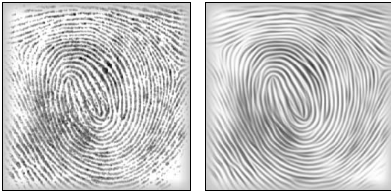
Fig. 4. Coherence-enhancing anisotropic diffusion of a fingerprint image. (a) LEFT: Original image, \Omega = (0, 256)^2 . (b) RIGHT: Filtered, \sigma = 0.5 , \rho = 4 , t = 20 . From [74].
