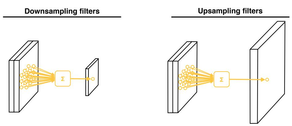
Upsampling filters allow to increase the resolution of the output Very useful to get full-resolution segmentation results
