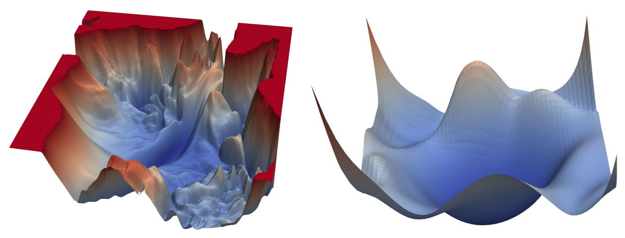
• The loss surface of a 56-layer net using the CIFAR-10 dataset, both without (left) and with (right) residual connections.
