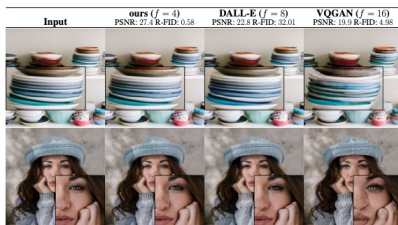
Figure 1. Boosting the upper bound on achievable quality with less aggressive downsampling. Since diffusion models offer excellent inductive biases for spatial data, we do not need the heavy spatial downsampling of related generative models in latent space, but can still greatly reduce the dimensionality of the data via suitable autoencoding models, see Sec. 3. Images are from the DIV2K [1] validation set, evaluated at 512^2 px. We denote the spatial downsampling factor by f . Reconstruction FIDs [28] and PSNR are calculated on ImageNet-val. [12]; see also Tab. 8.
