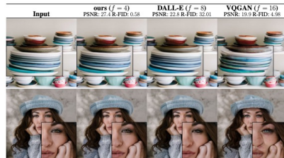
Figure 1. Boosting the upper bound on achievable quality with less aggressive downsampling. Since diffusion models offer excellent inductive biases for spatial data, we do not need the heavy spatial downsampling of related generative models in latent space, but can still greatly reduce the dimensionality of the data via suitable autoencoding models, see Sec. 3. Images are from the DIV2K [1] validation set, evaluated at 512^2 px. We denote the spatial downsampling factor by f . Reconstruction FIDs [28] and PSNR are calculated on ImageNet-val. [12]; see also Tab. 8.
