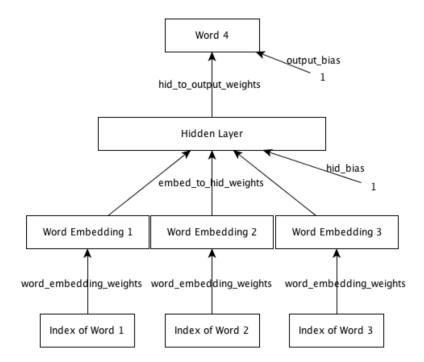
The network consists of an input layer, embedding layer, hidden layer and output layer. The input consists of a sequence of 3 consecutive words, given as integer valued indices. (*i.e.*, the 250 words
