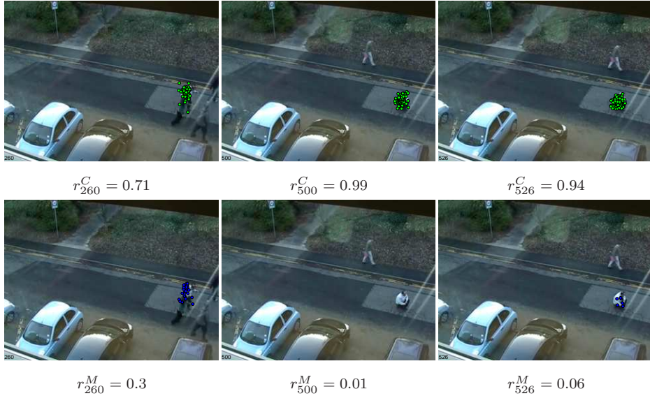
Figure 3: seq. 1 Visual representation of the cue reliabilities at three sample frames ( green for color and blue for motion).
