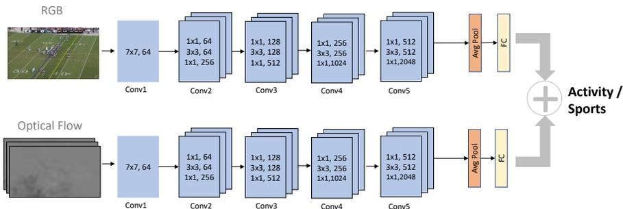
Figure 4: Two-Stream ConvNet architecture.
