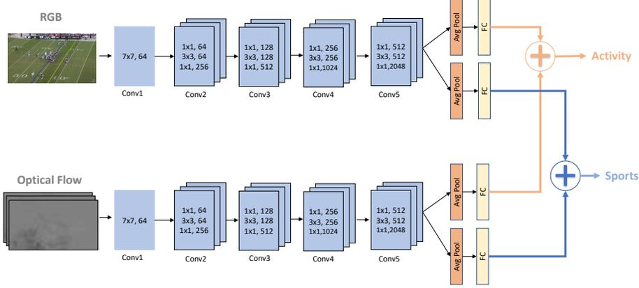
Figure 6: Multi-task version of Two-Stream ConvNet architecture.
