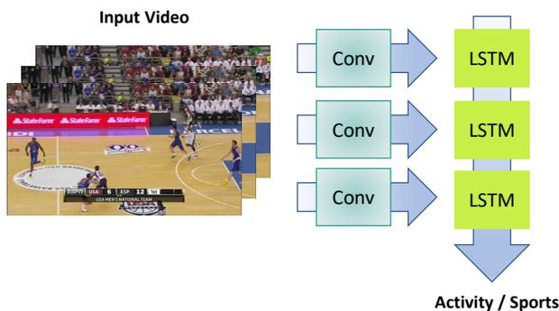
Figure 3: ConvNet + LSTM [19] model architecture.
