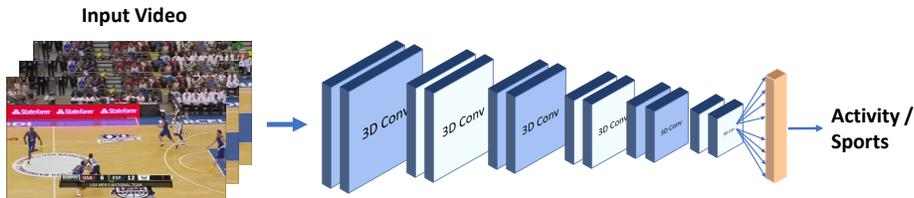
Figure 5: 3D ConvNet architecture.
