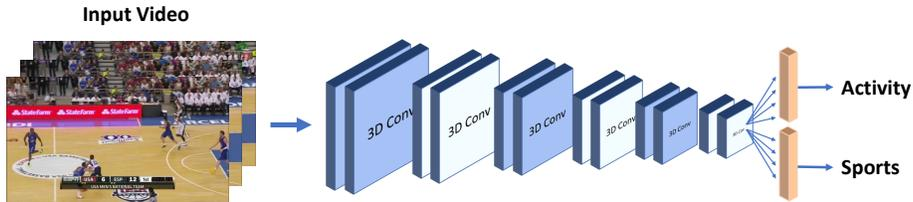
Figure 7: The Multi-task version of 3D ConvNet architecture.
