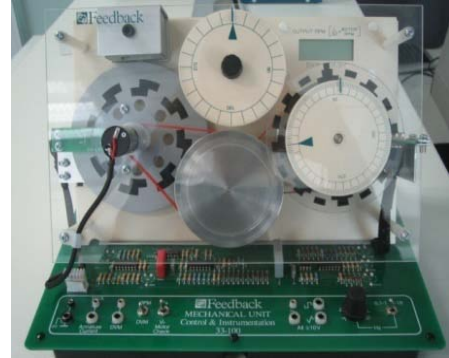
Figure 9: DC motor control setup.
