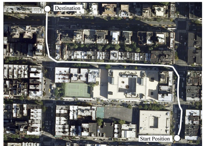
Fig. 14. Result of the fifth experiment. Variance threshold is 1.5 and a proper turn from a wide road to a narrow road is achieved after the start position. The vehicle then turns right to a wide road to approach the destination.
