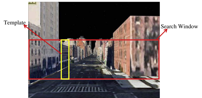
Fig. 4. Used search window and template in obstacle avoidance process.
