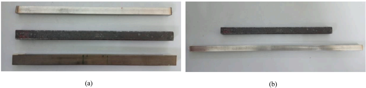
Fig. 6. Distributed-mass payloads used in the experiments (a) Different masses with same length, (b) Same mass with different lengths.
