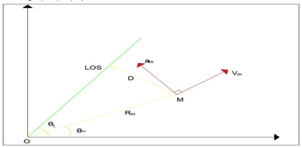
Figure 1: Kinematic model for target and missile positioned away from LOS  $a_m = KD$
