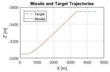
Figure 4.2: Missile and target trajectories using Dual FOPID controller.
