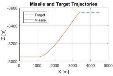
Figure 4.1: Missile and target trajectories using conventional PNG system.
