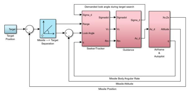
Figure 3.1: Conventional Guidance System
