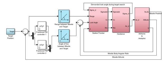
Figure 3.2: Dual Fractional Order PID Guidance System
