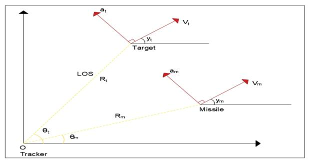
Figure 2: Kinematic model for missile and target with tracker
